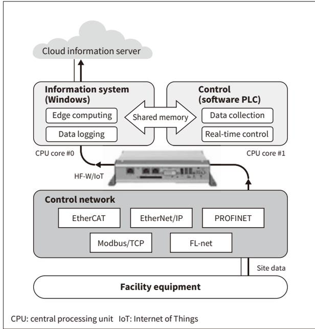
**Figure 5 — Block Diagram of HX Hybrid System**
