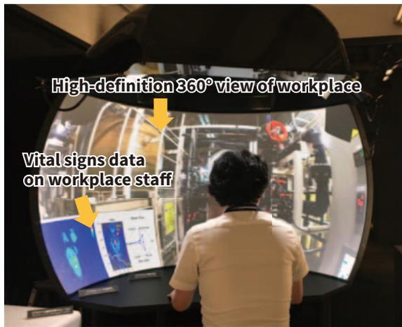
2 Prototype display for remotely located experienced workers
