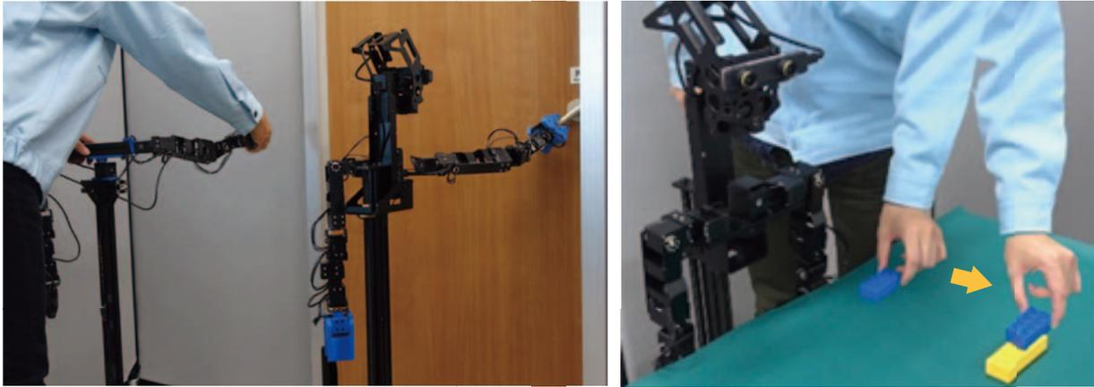
5 Teaching in progress using previous remote control method (left) and new imitation method (right)
