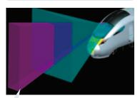
The front windscreen is designed to provide the driver's sightline that satisfies the requirements in UK standards while also reducing the size and weight of glass and making manufacturing easier
