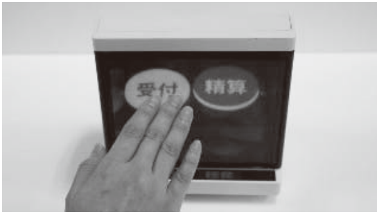
Non-touch Operation of Button Displayed by Compact Mid-air Input Device
