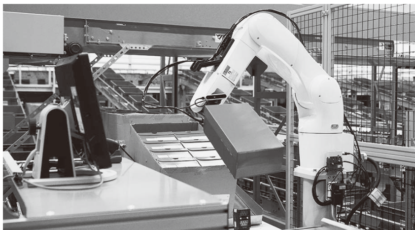
Figure 2 — Picking Robot Equipped with Autonomous Picking Robot System
