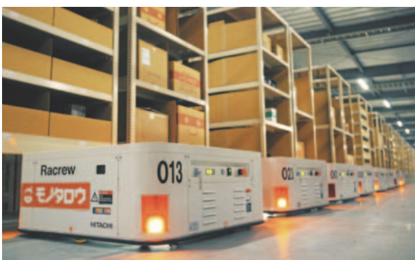
Figure 2 | Racrew, Compact Low-floor Automated Guided Robots in Operation at Kasama Distribution Center of MonotaRO Co., Ltd.
