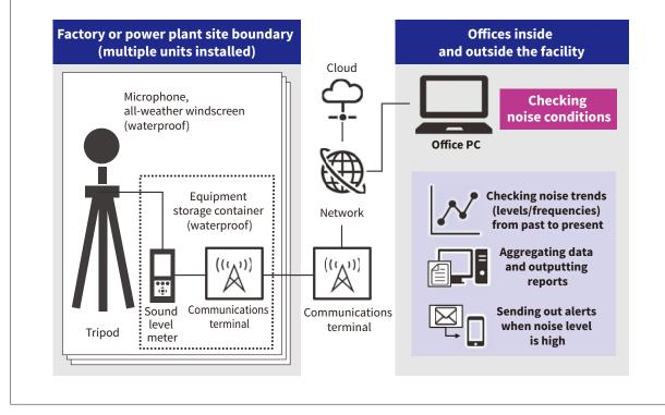
41 Equipment configuration of real-time noise monitoring system
