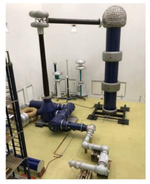
6 Dielectric type test of 420 kV passive elements in the highvoltage laboratory
