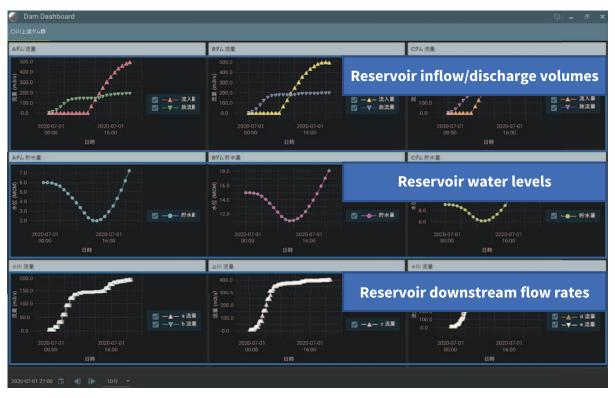
40 Screens displayed by the DioVISTA/Dam system for assisting reservoir operation
