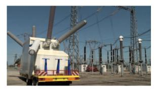
23 Modular mobile substation for disaster recovery
