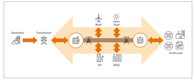
9 Bi-directional power-flow due to the renewable integrations in modern transmission and distribution grids
