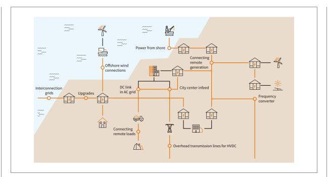
22 HVDC applications offer integration of renewables, interconnection of asynchronous grids between countries and regions and large scale power transmission with minimal losses
