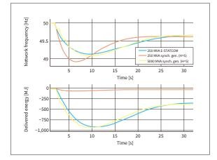
Comparison of synchronous generator (synch. gen.) and E-STATCOM providing synthetic inertia
