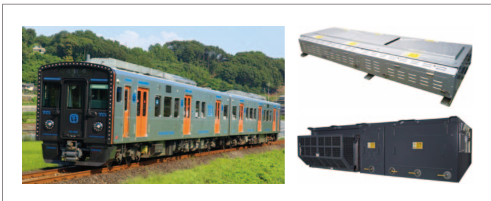
7 YC1 hybrid train of JR Kyushu (left), its storage batteries (top-right) and main converter (bottom-right)
