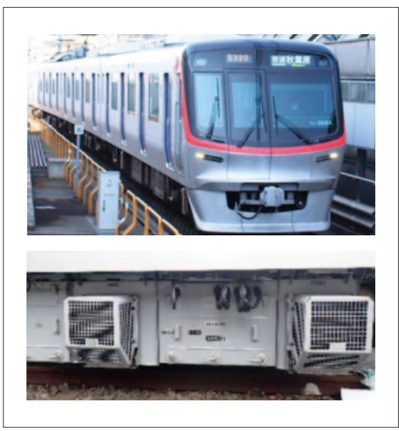
5 TX-3000 series train and its main converter
