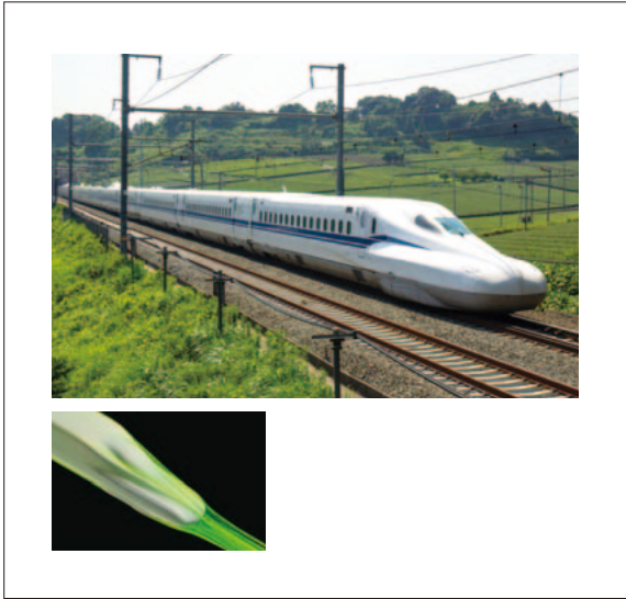
6 N700S Shinkansen train of JR Central and the result of fluid resistance analysis of the front shape
