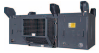
(b) VWF inverter unit (underfloor installation)
