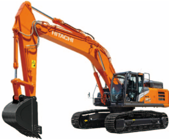
1 ZAXIS350LC-7 hydraulic excavator that meets European Stage V Standards
