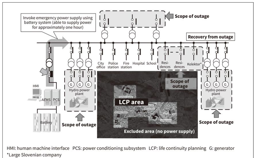
The designated LCP area is the area supplied by three medium- and high-voltage transformers installed at a substation in the Municipality of Idrija. Idrija experienced a power outage lasting several days in 2014 that was caused by ice and snow damage. It is also part of Alpine Town with a concept like that of environmental protection programs for the European Alps. As shown in **Figure 6**, the LCP area contains critical infrastructure, including a hospital and a police station.
