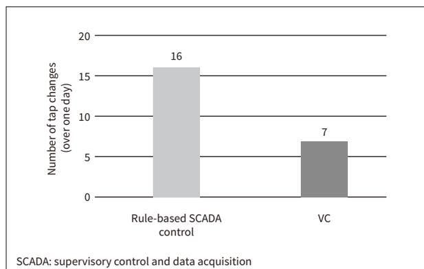
Furthermore, the comparison in **Figure 5** shows how VC required fewer tap changes to respond to voltage violations than the rule-based SCADA control technique used in the project by the Slovenian vendor, requiring only seven tap changes over the course of one day compared to 16 for rule-based SCADA control.
