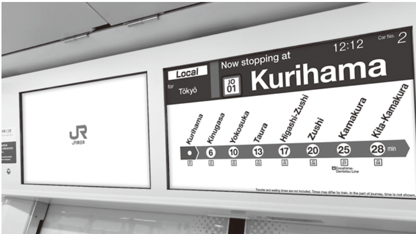
Figure 1 — On-board Passenger Information Display Installed over Door on Series E235 Rolling Stock of East Japan Railway Company (Yokosuka Line)
