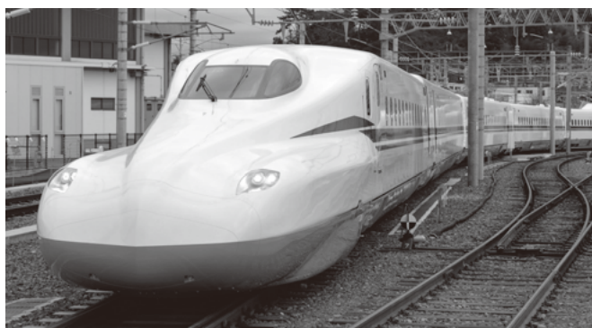
Figure 2 — Leading Shape of N700S Shinkansen
