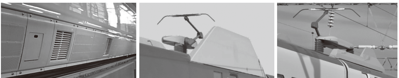
Figure 5 — Measures for Minimizing External Noise from Shinkansen
