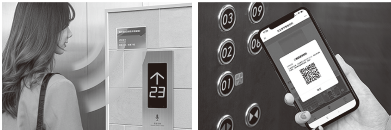
Figure 2 — Elevator Call Using Voice Recognition (Left) and Registration of Destination Floor with QR Code (Right)
