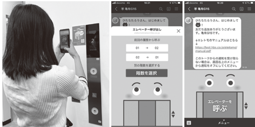
Figure 4 — LINE-linked Touchless Elevator Calling Service
