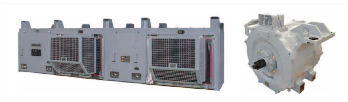
5 Inverter system (left) and main electric motor (right) used on the Fukutoshin Line 17000 series
