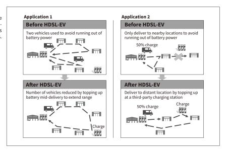
range by optimizing the charging schedule and choice of charger, also minimizing additional working time for drivers and their vehicles. This enables deliveries to proceed with no loss of efficiency as the number of destinations visited can be increased to the extent that the carrying capacity of the EV truck allows.
