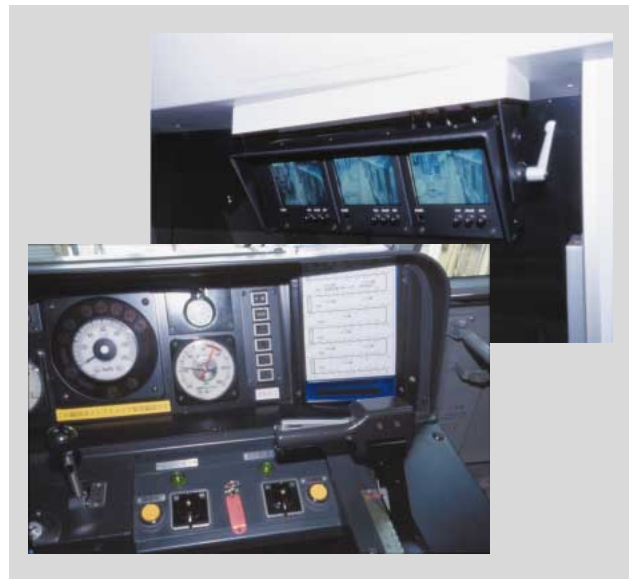
Fig. 6—One-person Operation of Trains on Tokyo Monorail Line.
