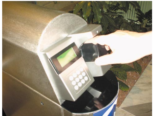
Fig. 8—Gate Equipped with Finger-vein Scanner. The entrance gate is fitted with an authentication scanner.
