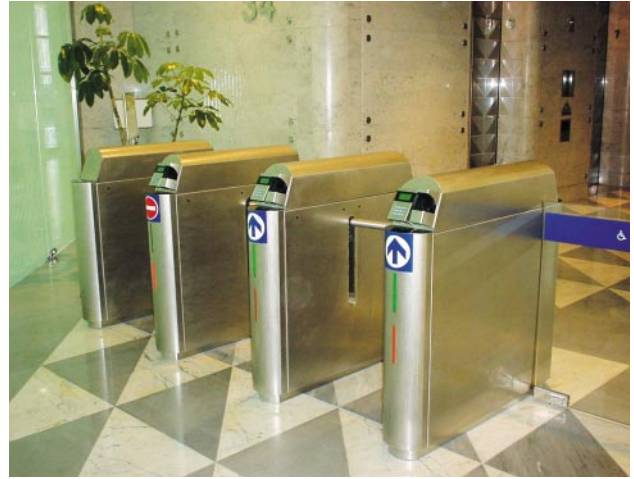
Fig. 7—Finger-vein-authentication System for Office Building. About 1,500 persons are enrolled in this system.
