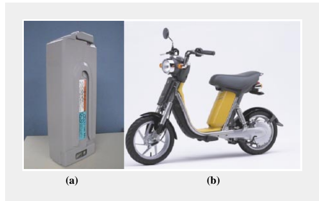
Fig. 5—Lithium Battery Module for Light Vehicles (a) and Yamaha Motor Co., Ltd.'s Electric Motor Scooter (b). This compact sized module with 26 V and 14 Ah can power this light vehicle run at around 30 km. The module can be charged to 80% in one hour with a specially developed battery charger operated by 100-V AC supply.
