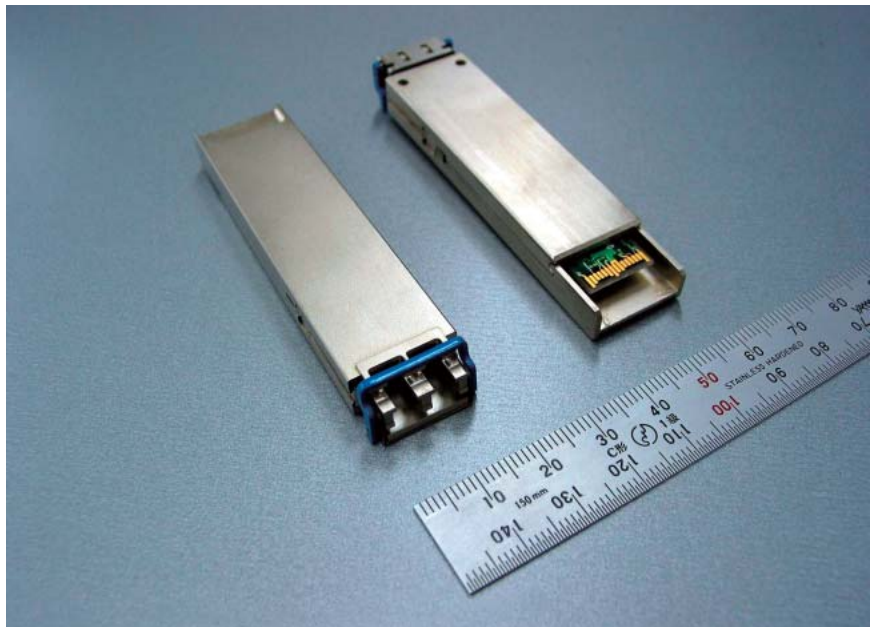
XFP MSA compliant compact-size 10-Gbit/s optical transceiver modules
