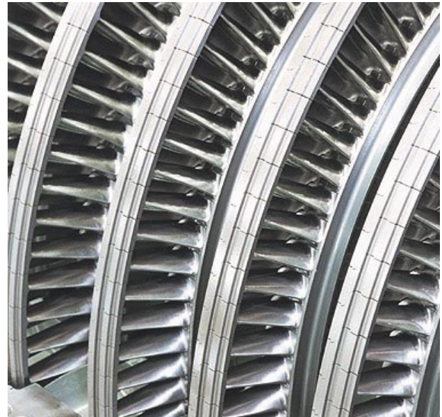
Fig. 4—High-pressure Turbine Blades with CCB. Blades are interconnected by tip covers.
