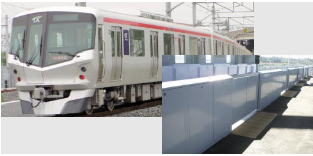
Fig. 11— Tsukuba Express Car and Platform Gate. TX-2000 series cars (left) and platform gates to support safe driver-only operation (right).
