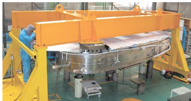
Fig. 8—Photo of Partially Assembled Equipment at the Plant. To reduce the on-site installation work, completed sector magnet components were partially assembled at the plant before delivery to the site.
