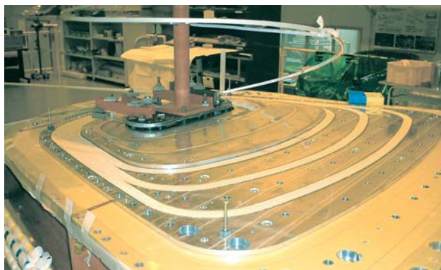
Fig. 7—SC Trim Coil Winding. The block construction Al alloy coil support assemblies and unique and double pancake windings are alternately assembled.
