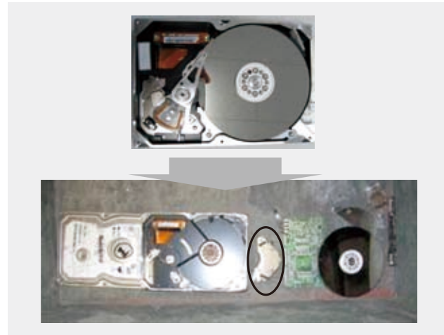
Fig. 8—HDD Dismantling (Showing Results of Dismantling).
