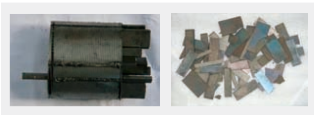
Fig. 7—Recovery of Magnets from Rotor.
