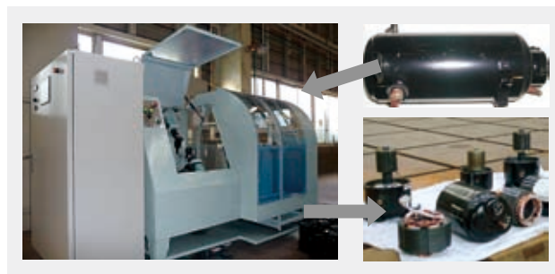
Fig. 4—Compressor Dismantling Machine. This is the machine for automatically cutting off the steel shell.
