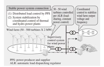
Fig. 6—Wind Farm Control System. Hitachi has drawn on its expertise in conventional power systems to stabilize wind-generated power.
