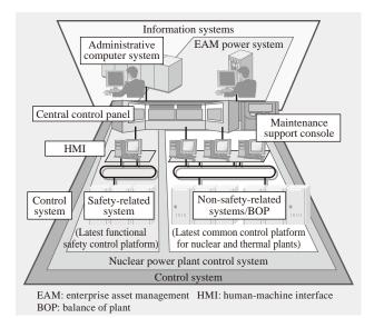
*Fig.* 4—*Concept behind Control System for New Nuclear Power Plants.*
