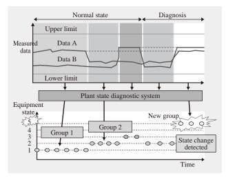
Fig. 7—Plant Diagnosis System. ART (adaptive resonance theory) allows user-friendly plant diagnosis.
