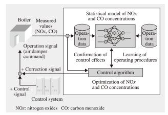
Fig. 3—Configuration of Control System for Reducing Environmental Impact.
