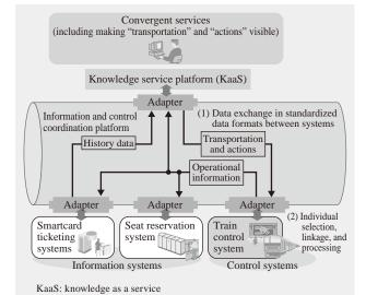
Fig. 3—Convergence of Information Systems and Control Systems in System Architecture for Services. Knowledge processing of huge amount of data can be achieved using an "information and control coordination platform" to provide loosely coupled coordination of various information and control systems together with a "knowledge service platform."
