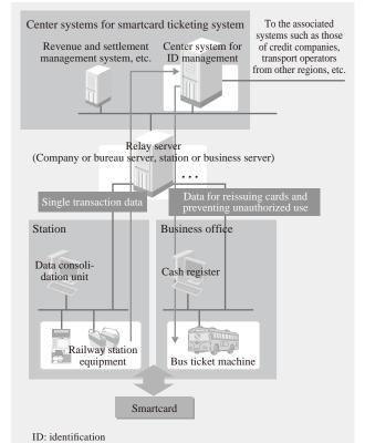
Fig. 3—Overview of Smartcard Ticketing System. Data on smartcard use (itemized transaction data) is sent from terminals to the center system and the accumulated data used for reissuing cards and preventing unauthorized use.
