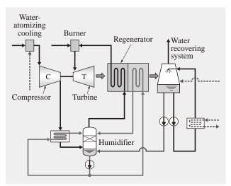
Fig. 4—AHAT System Diagram. AHATs (advanced humid air turbines) achieve efficiency similar to combined cycle using a standalone gas turbine.
