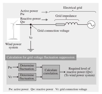
*Fig.* 5—Use of Reactive Power to Suppress Grid Voltage Fluctuation.
