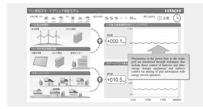
Fig. 6—Example Screen from Rokkasho Village Smart Grid Demonstration in Aomori Prefecture. In addition to power flow monitoring, voltage and current monitoring, and smart house demand and supply monitoring, the project also includes the control of energy storage based on monitoring and forecasting of demand and the level of renewable generation.
