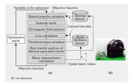
Fig. 5—Flow Chart of Coupled Thermal and Magnetic Field Analysis (a) and Hitachi's First Electric Motor Next to a Prototype Motor (b). The prototype motor is approximately onefifteenth the size of Hitachi's first electric motor [a 5-HP (horsepower) induction motor, Hitachi's first ever product].
