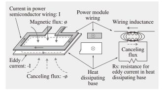
*Fig. 3—Technique for Reducing Inductance of Power Module Wiring.*
