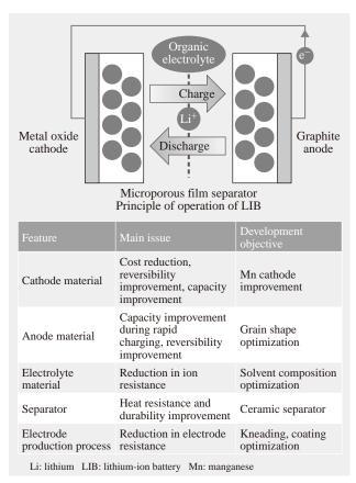
*Fig.* 4—*Principle of Operation of LIB and Development Objectives.*
