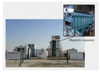
Fig. 6—Red Tide Removal System Installed in the Gulf Coast of the Arabian Peninsula. The plant has a capacity of 400 m<sup>3</sup>/h and is installed in four 20-foot containers for ease of transport.
