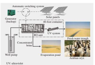
Fig. 3—Flow Chart of Solar RO System. Salt-contaminated groundwater is pumped up and then desalinated in the RO units to produce fresh water. Photovoltaic generation provides the operating power.
