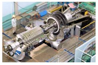
Fig. 8—Cutaway Photograph of 40-MW-class AHAT Gas Turbine. Tests are scheduled to commence from the latter half of the 2011
