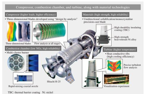
Fig. 7—Gas Turbine Research and Development Examples. To improve efficiency and reduce the environmental burden, Hitachi is working on a broad range of research and development covering the compressor, combustion chamber, and various material technologies, as well as the turbine unit itself.
