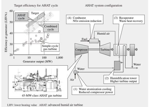
Fig. 9—AHAT System Configuration and Efficiency. The aim for the AHAT system is to achieve an efficiency equal to or better than that of a combined cycle plant despite using only a gas turbine.
