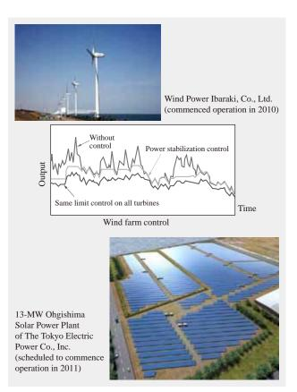
Fig. 14—Renewable Energy Generation System and Interconnection Technology. Hitachi supplies interconnection technology that helps with
