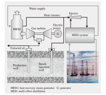
*Fig. 10—Trigeneration System Producing Electric Power, Heat, and Water.*
