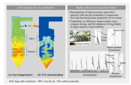
Fig. 6—Example Research and Development of Coal-fired Thermal Power Plants (Boilers and Steam Turbines). Hitachi is using numerical simulation to develop products, such as low-NOx burners and highly efficient supercriticalpressure steam turbines.
