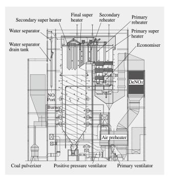
Fig. 6—Side Elevation Drawing of Torrevaldaliga Nord Boiler. A design function evaluation of the main pressurized components was undertaken by Hitachi Power Europe GmbH to ensure compliance with European standards for boiler materials.
