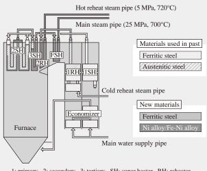
1: primary 2: secondary 3: tertiary SH: super heater RH: reheater FSH: final super heater
