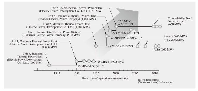
Fig. 4—Evolution of Steam Conditions of Plants Supplied by Babcock-Hitachi K.K. Hitachi has built up experience with high-capacity plants that use supercritical or USC power generation.
