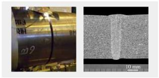
Fig. 11—Boiler Welding. Testing involving narrow-groove HST [hotwire switching TIG (tungsten inert gas)] welding of HR6W Ni alloy has demonstrated the integrity of the welds.
