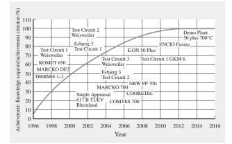
Fig. 12—European Research and Development Programs for 700°C-class Technology. Sufficient knowledge has been acquired to construct a demonstration plant in the near future.
