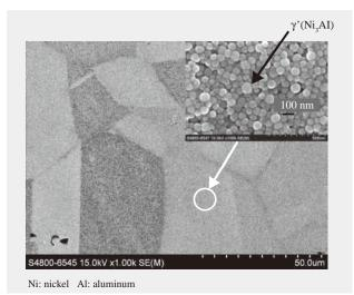
Fig. 7—The new Ni-Fe base superalloy Microstructure. This photograph taken by a scanning electron microscope shows the presence of a precipitation-hardened Ni<sub>3</sub>Al phase in the new Ni-Fe base superalloy.
