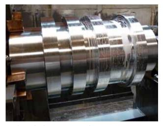
Fig. 9—Study of A-USC Rotor Production. Since the Ni alloy to be used for A-USC has higher strength than previous steels, research and development of its machinability is also important.
