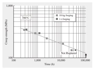
Fig. 8—Long-term Creep Testing of the New Ni-Fe Base Superalloy.
