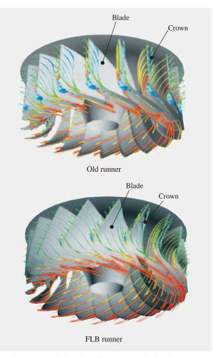
Fig. 4—Patterns of Flow through Runners Calculated Using CFD. The figure shows the patterns of flow through the runners (with the band removed). On the old runner, the flow becomes detached in the inlet region and is biased toward the band end. In the FLB runner, in contrast, the flow in the inlet region is smooth and extends to the crown end without being biased toward the band end.
