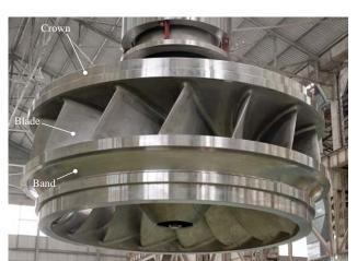
Fig. 5—FLB Runner. The photograph shows the FLB runner prior to delivery from the factory. It has an outlet diameter of about 1 m and 15 blades.
