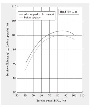
Fig. 3—Verification of Characteristics Improvements Using CFD. Adopting FLB runners (thick line) improved efficiency by 1.5 to 2% over the entire operating range compared to before the upgrade (thin line).
