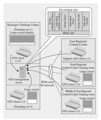
Fig. 3—Block Diagram of OTS. The training sites connect via wide-area IP network to the simulation server located at the Kawagoe Training Center.
