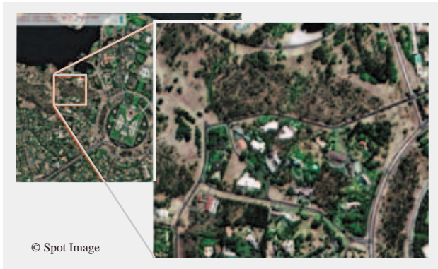
Fig. 3—Satellite Images of Forest Area. These images (of Canberra, Australia) with 2.5-m resolution were taken by the French SPOT satellite. They can be used to determine the presence or absence of forest, the types of trees (species), and the forest area.
