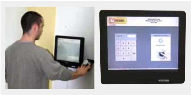
Fig. 2—Attendance Management System in Use (Left) and Example Screen (Right). After performing a simple set of operations on the touch panel PC (personal computer), the user places their finger on the scanner to record attendance information.
