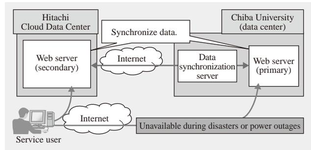
Fig. 8—Example Use of Cloud for Information Distribution at University during Disaster or Power Outage (Chiba University). Chiba University uses a hybrid cloud that links the web servers at its own data center to servers at Hitachi Cloud Data Center to cope with disasters or power outages.
