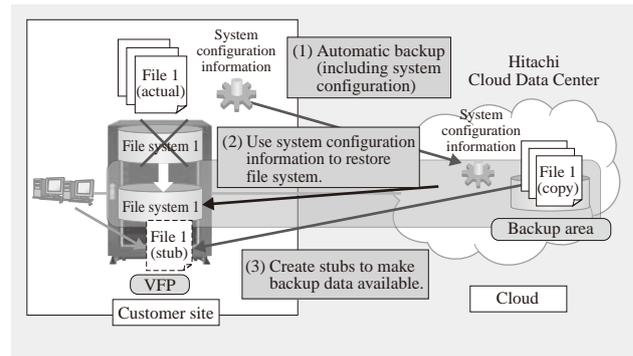
Fig. 6—Overview of Managed Service for Backing up File Storage System.
