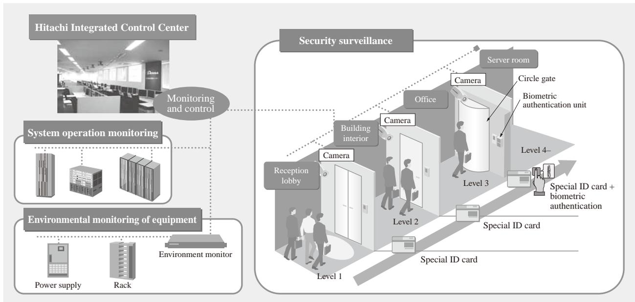
Fig. 10—Technologies and Products for Achieving High Level of Security. A high level of security is achieved using measures such as centralized monitoring, circle gates, and biometric authentication.
