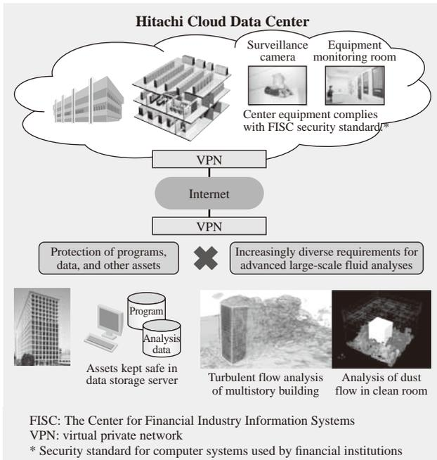
Fig. 7—Overview of Fluid Analysis System of Kajima Corporation.
