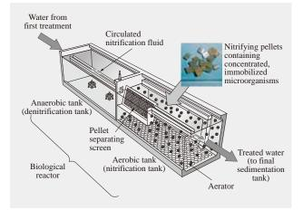
Fig. 4—Immobilized Microorganism Treatment System. Processing time can be halved by using nitrifying pellets that contain nitrification reaction bacteria.
