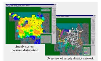
*Fig.* 6—*Example Screen from Water Distribution Control System. The system manages the pipe network in the district being supplied and predicts the pressure distribution.*
