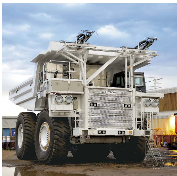
Fig. 9—EH3500ACII Trolley-assisted Dump Truck. This EH3500ACII trolley-assisted dump truck was supplied to a copper mine in the Republic of Zambia in Africa.
