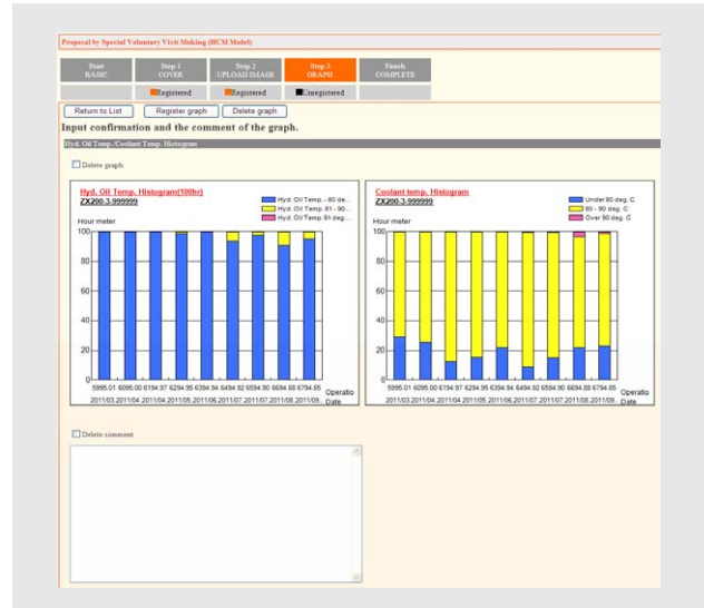
Fig. 4—Example Repair Proposal Screen. Convincing proposals can be produced by combining operational data with the results of a visual inspection.
