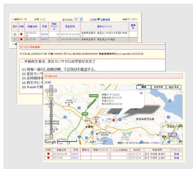
Fig. 6—Example Screens for Event Monitoring System. The screens present engine status information together with guidance on what to do next based on events from the machine.
