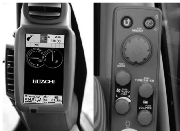
Fig. 7—Multi-function Monitor and Controls. The photographs show the main screen of the multi-function monitor (left) and the multi-function switch and air conditioning and radio switches (right).
