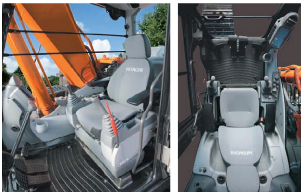
Fig. 5—ZAXIS-5 Series Cab Interior. The spacious and comfortable cab improves monitor visibility and the right-hand-side field of view.
