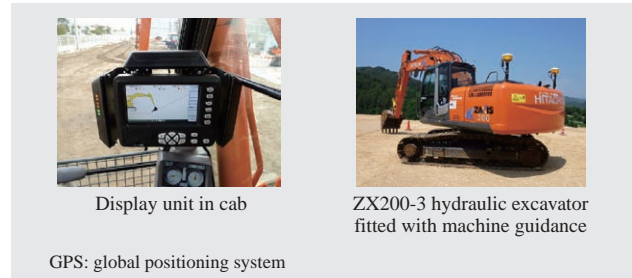
Fig. 6—Information-integrated Construction Machinery. The photographs show a construction information display unit (left) and an information-integrated construction machine (right). The two masts are GPS receivers.
