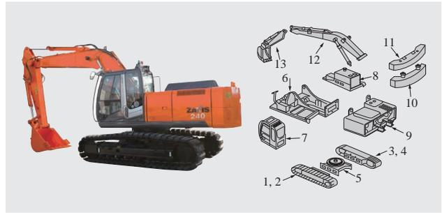
Fig. 9—1.0-m<sup>3</sup>-class Disassemblable Hydraulic Excavator in Assembled and Disassembled Forms (Excluding Accessories). The design includes use of flanges on detachable parts of structural components, one-touch hydraulic couplings, electrical connectors, and a weight that can be split into upper and lower halves.
