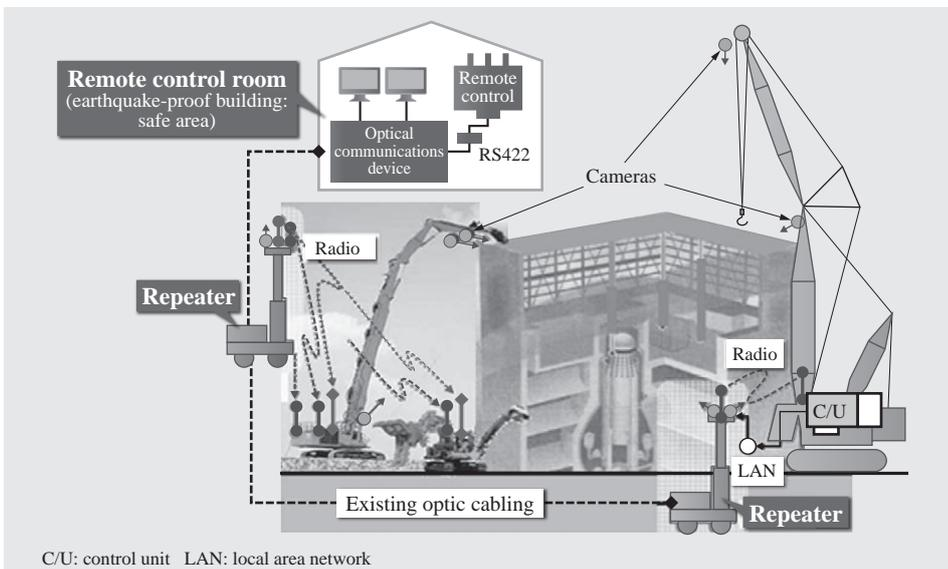
Fig. 7—Proposed Remote Control System for Large Machinery. Hitachi Construction Machinery was quick to propose a remote control system using equipment such as demolition machines and large cranes to the relevant authorities, and started work on preparing the machinery and radio control system.
