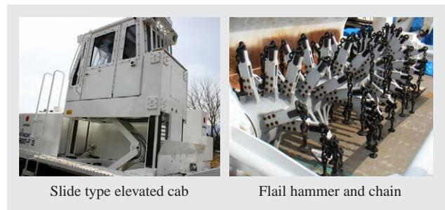
Fig. 4—Slide Type Elevated Cab, and Hammer and Chain. The cab is located at the rear of the machine for safety, and the hammers and chains are designed to allow refurbishment by local technicians to repair any wear or damage.
