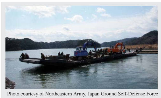
Fig. 6—Use of Type 92 Floating Bridge in Recovery Work. The floating bridge was used to transport construction machinery needed for recovery work to an island cut off by the Great East Japan Earthquake.
