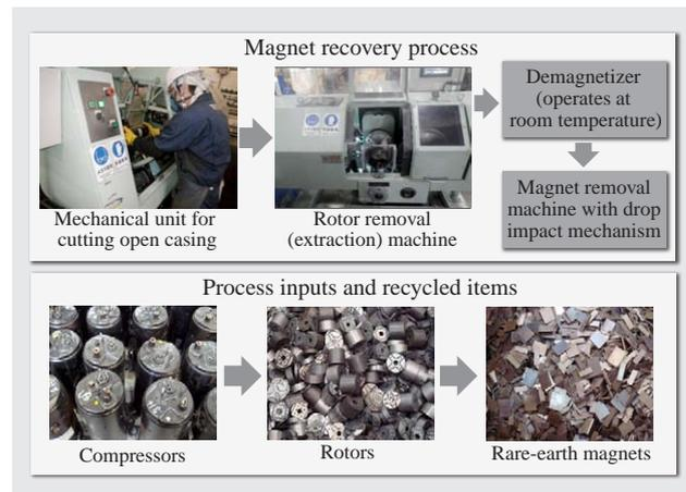
Fig. 3—Process Used to Separate and Recover Rare-earth Magnets from Air Conditioners.
