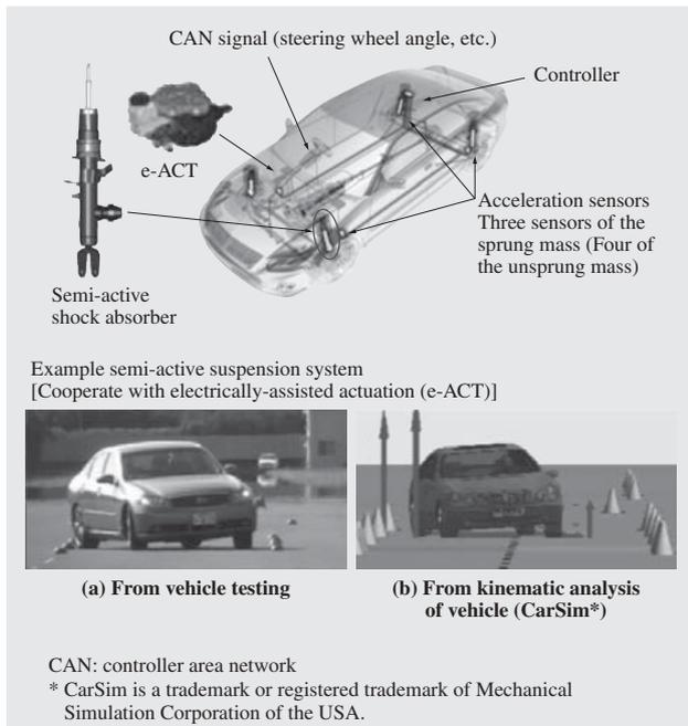
Fig. 6—Cooperative Control System for Semi-active Suspension and Controlled Brake. Cooperative control of the semi-active suspension and brake (e-ACT) can improve vehicle stability when taking evasive action.
