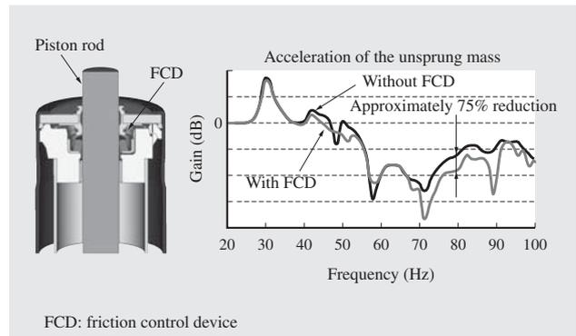
Fig. 7—Structure and Benefits of FCDs. Fitting FCDs significantly reduces high-frequency vibrations of the unsprung mass with major benefits for ride comfort.
