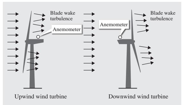
Fig. 3—Location of Anemometer and Relationship with Blade Wake.
