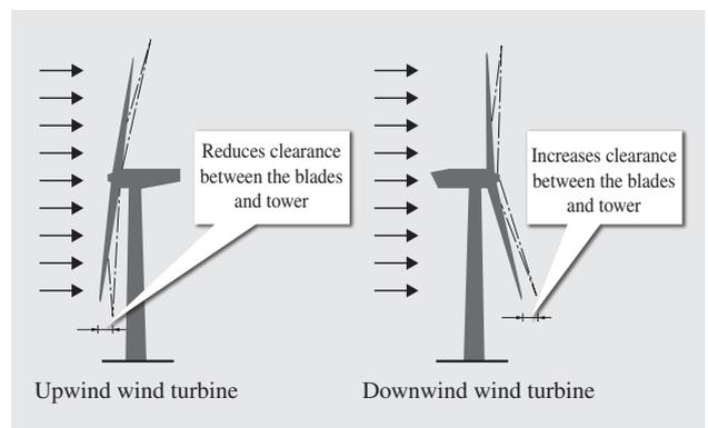
Fig. 4—Clearance between the Blades and Tower during High Winds.
