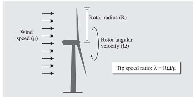
Fig. 6—Wind Turbine Tip Speed Ratio.
