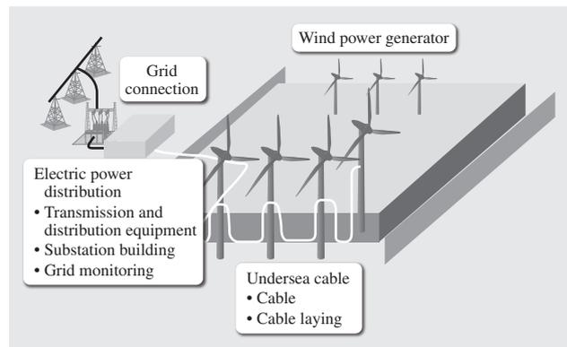
Fig. 7—Overview of Electric Power Distribution Equipment.
