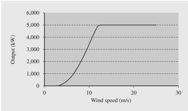
Fig. 2—Design Power Curve.
