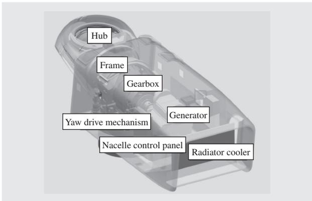
Fig. 5—Equipment Layout in Nacelle.
