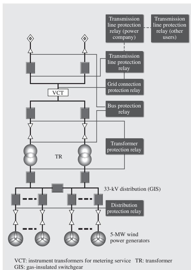
Fig. 8—Connection Diagram for Substation Equipment for Connection to Grid (Overview).
