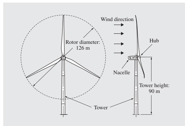
Fig. 1—Overall Dimensions of HTW5.0-126.
