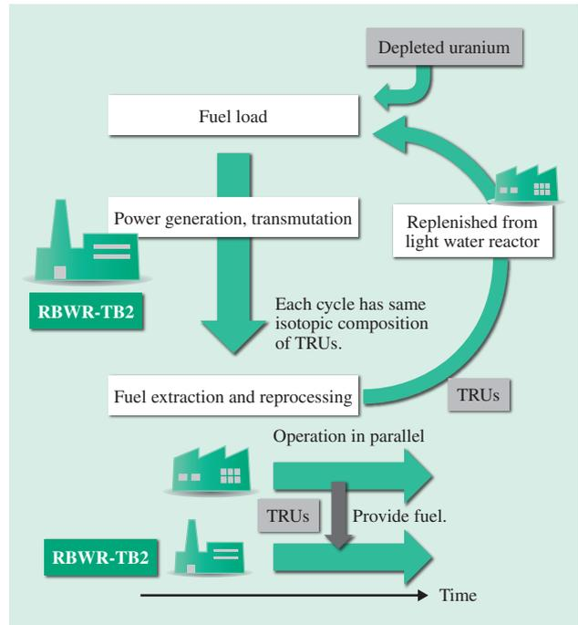
Fig. 5—Fuel Cycle for RBWR-TB2. The TRUs consumed during operation are replenished from the spent fuel of light water reactors. The RBWR-TB2 operates in parallel with a light water reactor to minimize the buildup of excess TRUs.
