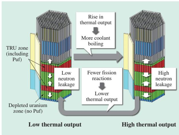
Fig. 2—Inherent Safety of RBWR.
