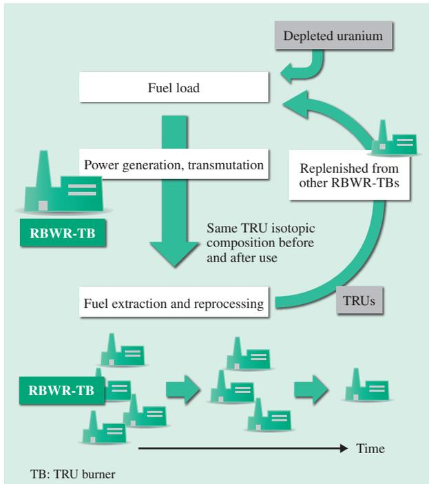
Fig. 4—Fuel Cycle for RBWR-TB. The TRUs consumed during operation are replenished from the spent fuel of other RBWR-TBs. The fuel is recycled through progressively fewer reactors until all the TRUs are burned up apart from those in the final reactor.
