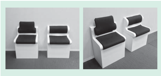
Fig. 3—Mockup of UD Seat. Hitachi is developing UD seats for use in trains.
