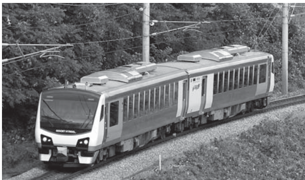
Fig. 9—Series HB-E300 Resort Train. 15.2 kWh of lithium-ion batteries are installed on top of each car.
