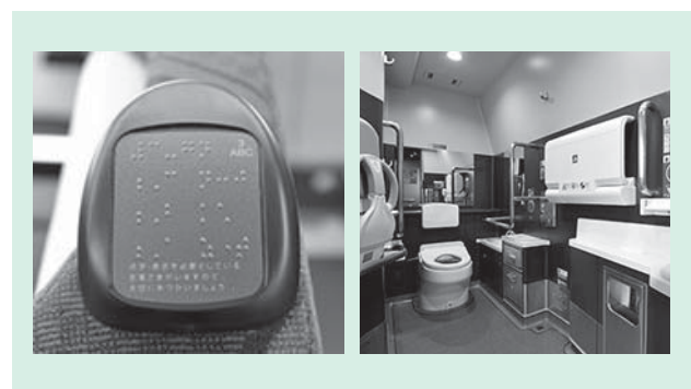
Fig. 2—Braille Signage and Multi-function Toilets for Latest High-speed Shinkansen Rolling Stock. The latest high-speed Shinkansen rolling stock use internal fittings selected with barrier-free accessibility in mind.
